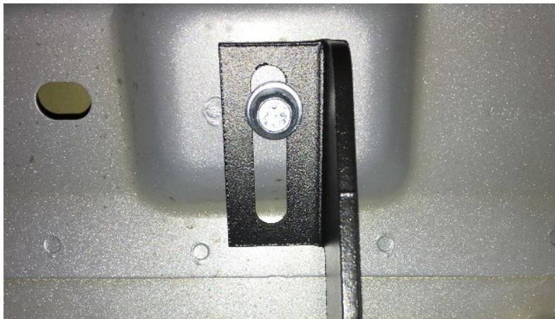
**Step. 5** Next, start all (x6) ¼"-20"x 3/4" hex bolts, (x12) M8 flat washers, (x6) 5/16" lock washers and (6) ¼"-20 HC Nut in the pinch weld mounting locations and leave loose for now.
