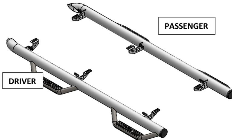
**Step 2:** Depending on your cab model, you will have to identify which hardware you will have to use for the upper (3) mounts on the underside of the body. There will either be existing 8mm threaded holes for the M8 x 20mm hex head bolts or open slots for the 3/8" speed clips and 3/8"x 1 1/4" Hex bolts.
