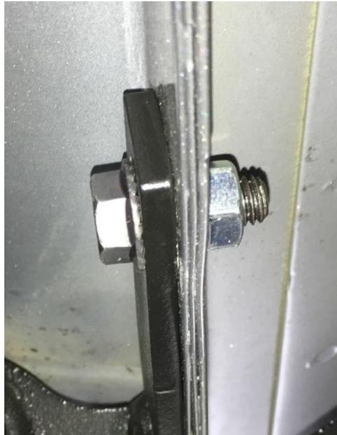
**Step. 6:** After final positioning, completely tighten all (x6) ¼"-20 x ¾" in the pinch weld attachment.
